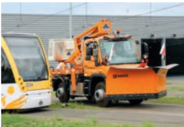
On road or rails: a snow plough is fitted for winter service operations in a matter of minutes
