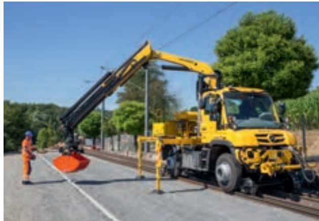
Flexible track construction vehicle for infrastructure work and pulling wagons
