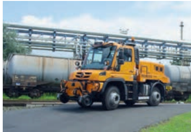
Fast changeover: a level stretch of track covering just a few metres is sufficient for rail/road changeover
