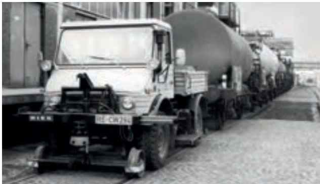
Already in service as a shunting vehicle back in the 1960s: Unimog U 406 with special tyres
