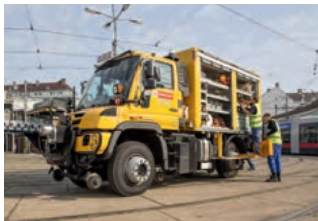
Rerailing derailed wagons with the aid of a Unimog rescue vehicle
