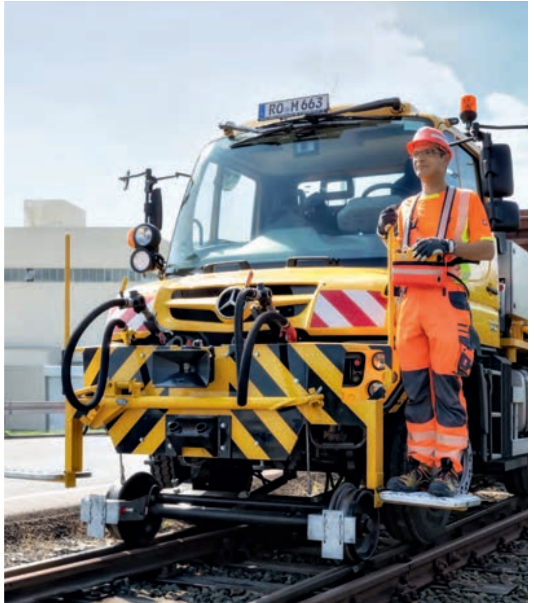
Coupling up, then shunting: by means of radio remote control the line of wagons can be controlled from the front end of the train at all times in one-man mode
