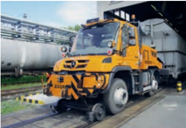
Pulling power for up to 1000 t: Unimog in shunting operation
