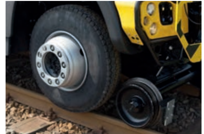
Ample pulling power: the Unimog wheels provide the necessary traction – enabling the Unimog to tow loads of up to 1000 t
