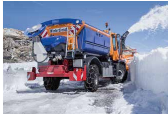
Turning the corner - with all-wheel steering: the auxiliary rear axle steering gives the Unimog even greater manoeuvrability.
