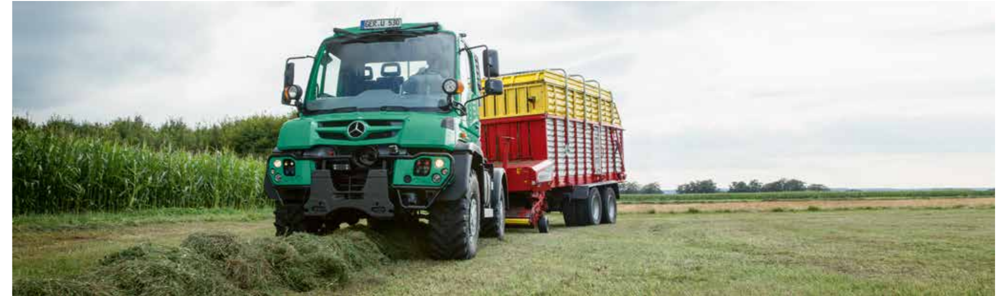
Portal axles ensure good ground clearance – e.g. when working with a forage wagon.
