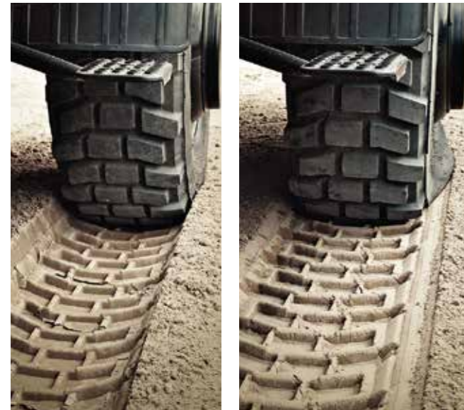
The central tyre inflation system (CTIS) can be activated from the steering wheel – even while the vehicle is moving.
