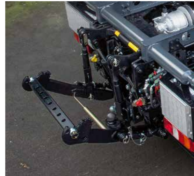
Height-adjustable trailer coupling with 80 mm ball and rear power lift with up to 5 t hoisting power.
